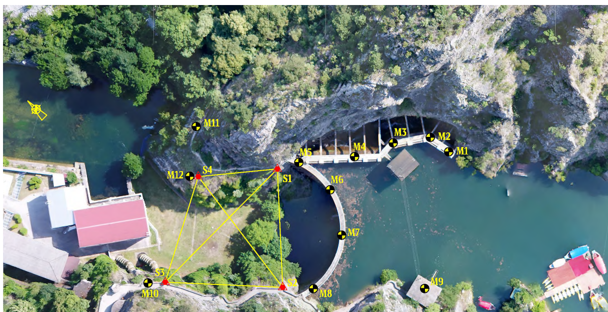
Figure 4: Geodetic network with layout of orientation points
