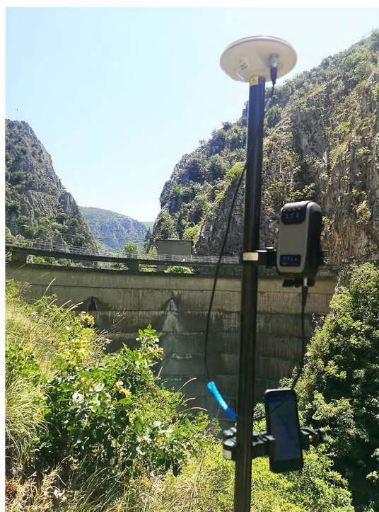
Figure 2: GNSS positioning of the points from the microtrigonometric network of the dam
