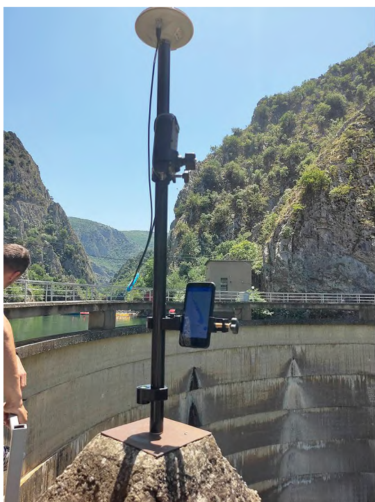
Figure 2: GNSS positioning of the points from the microtrigonometric network of the dam
